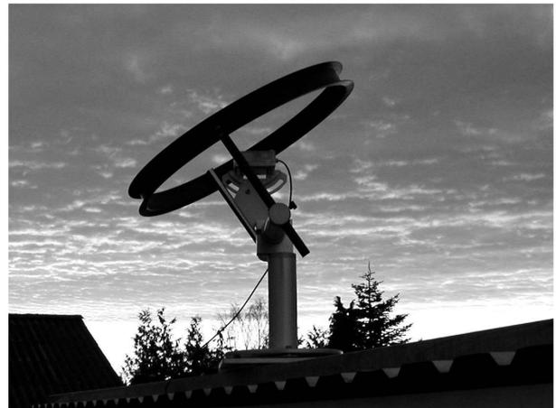
**Figure 1:** A shadow ring and pyranometer are used for measurement of the diffuse solar irradiance.
