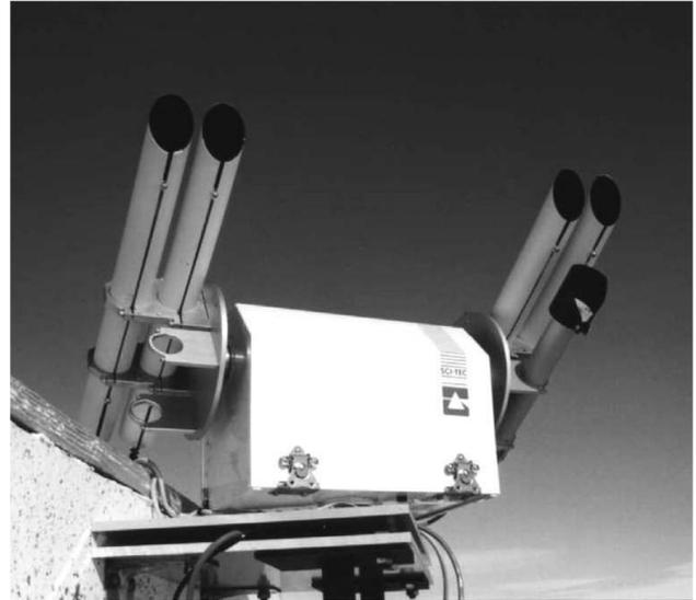
**Figure 2:** Tracker with pyrheliometers used to measure direct solar irradiance  $I_D$  in northern Greenland (76,5° N) [2].
